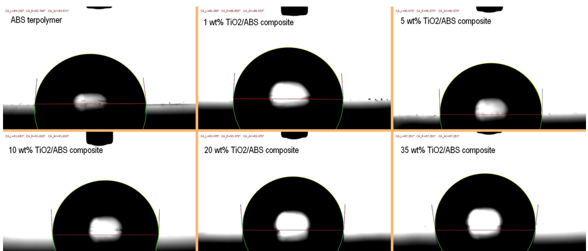
Figure 9. The images of the sessile water drop on the surface of TiO 2 /ABS composites
