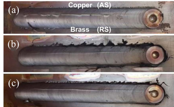
Figure 4. Surface images of lap joints between copper and brass alloys in case A with the condition of (a) 450 rpm- 16 mm/min (b) 710 rpm- 25 mm/min (c) 710 rpm- 16 mm/min
