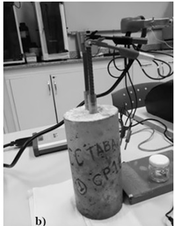
Figure 2. Electrochemical measurements - cylindrical concrete blocks, (a) upper view and (b) front view.
