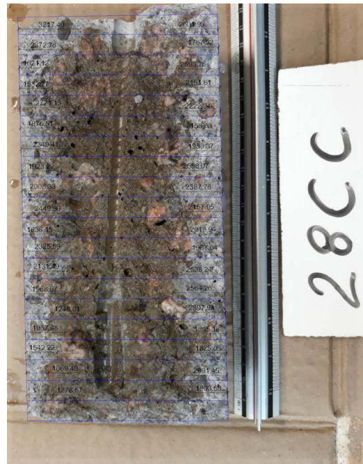
Figure 13. Chloride Penetration of samples with 28-day curing for 40 cycles.
