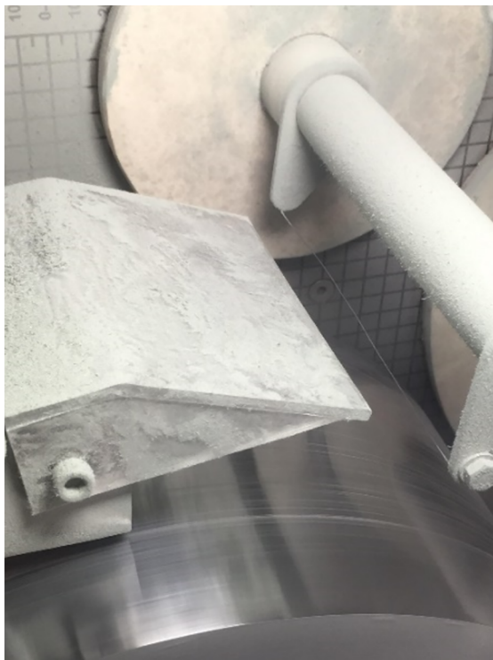
Figure 4. PCB dust accumulation in electrodes.
