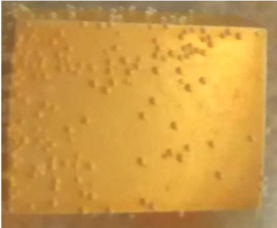
Figure 4. AZ91D alloy during cerium conversion coating bath with hydrogen evolution.
