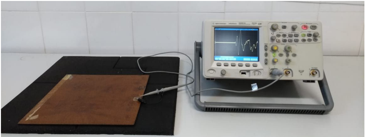
Figure 2. The perspective view of the testing system of sensors based on 1-3 PUR/PZT piezoelectric composite.
