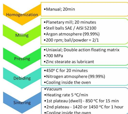
**Figure 1.** Powder Metallurgy processing parameters of the NbC-7.5Ni-7.5(Ni-12Al) cermet.
