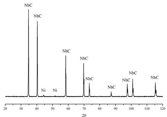
**Figure 5.** XRD pattern of the NbC-7.5Ni-7.5(Ni-12Al) cermet sintered at 1420 °C.
