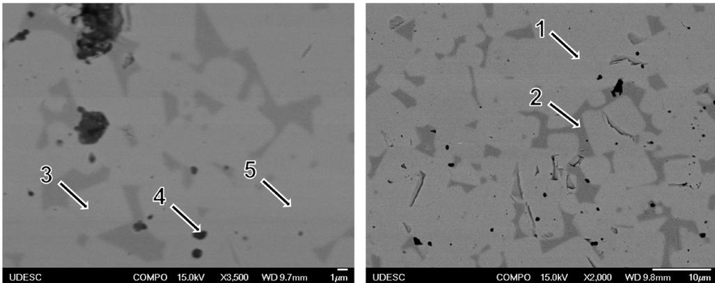
**Figure 7.** SEM – BSE image of NbC-7.5Ni-7.5(Ni-12Al) cermet sintered at 1420 °C. 1, 3 and 5 – NbC, 2 – (Ni), 4 – Pore.
