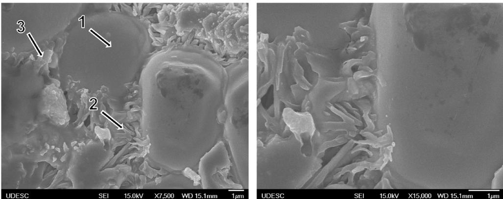
**Figure 8.** SEM – SE image of NbC-7.5Ni-7.5(Ni-12Al) cermet surface sintered at 1420 °C. 1 - Polygonal NbC particles, 2 and 3 - Branches of the binder.
