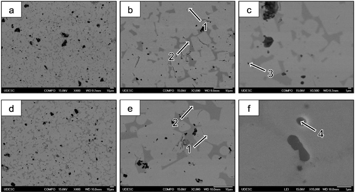
**Figure 6.** SEM – BSE images of the NbC-7.5Ni-7.5(Ni-12Al) cermet sintered at 1420 °C (a-c) and 1450 °C (d-f). 1 - NbC, 2 – (Ni), 3 - Al<sub>2</sub>O<sub>3</sub>, 4 - Pores.
