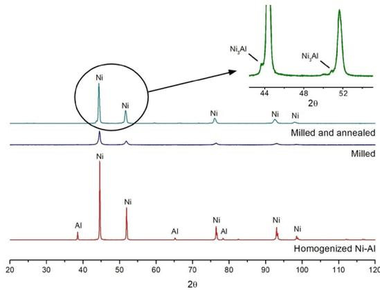
**Figure 2.** XRD patterns of Ni and Al powder mixtures after different processing stages to obtain Ni-12Al (wt%).
