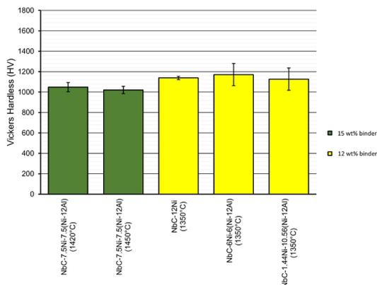
**Figure 9.** Hardness of NbC cermets.
