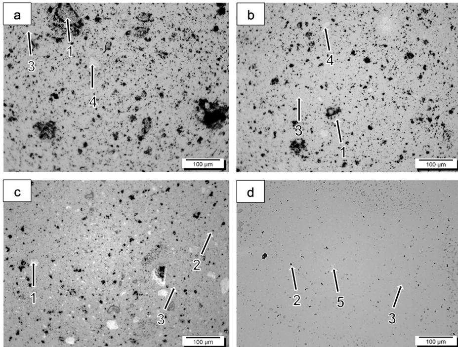
**Figure 4.** Optical microscopy images of NbC cermet with 12 wt% binder sintered at 1350 °C: (a) NbC-1.44Ni-10.56(Ni-12Al), (b) NbC-3Ni-9(Ni-12Al), (c) NbC-6Ni-6(Ni-12Al) and (d) NbC-12Ni (wt%). 1 – Agglomerates, 2 – pores, 3 – NbC, 4 – (Ni), 5 – Ni.
