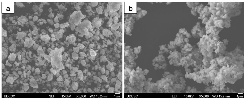
**Figure 3.** SEM – SE image of morphology of the Ni-12Al (wt%) powder mixture in (a) milled and (b) milled and annealed conditions.
