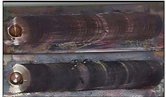
**Figure 10.** Test specimens welded with  $\Omega$  950 rev.mm<sup>-1</sup> and  $v$  20 mm.min<sup>-1</sup>.
