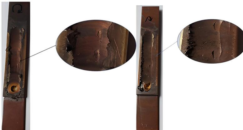
**Figure 12.** Welded samples with parameters  $\Omega 850 \text{ rev.mm}^{-1}$   $\mathbf{v} 60 \text{ mm.min}^{-1}$  and  $\Omega 850 \text{ rev.mm}^{-1}$   $\mathbf{v} 20 \text{ mm.min}^{-1}$  respectively, defects in details.
