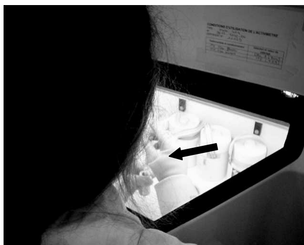
Figure 1 - Dispensing procedure in PET workstation (arrow points out drawing up of tracer)
