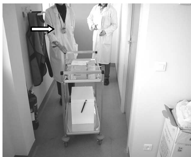
Figure 2 - Example of positioning of the electronic dosimeter during the transportation of shielded syringe
