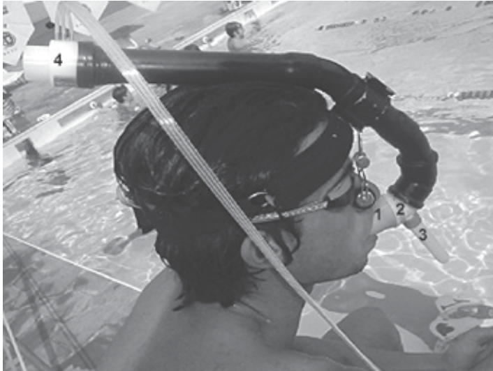
Figure 1 – Representation of the Snorkel developed for measurement of cardiorespiratory parameters in swimming
