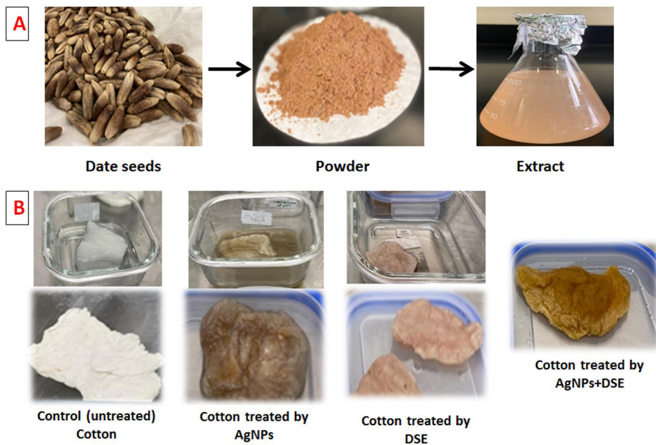
Figure 1. (A) Formation of DSE, (B) preparation of treated cotton fabrics.
