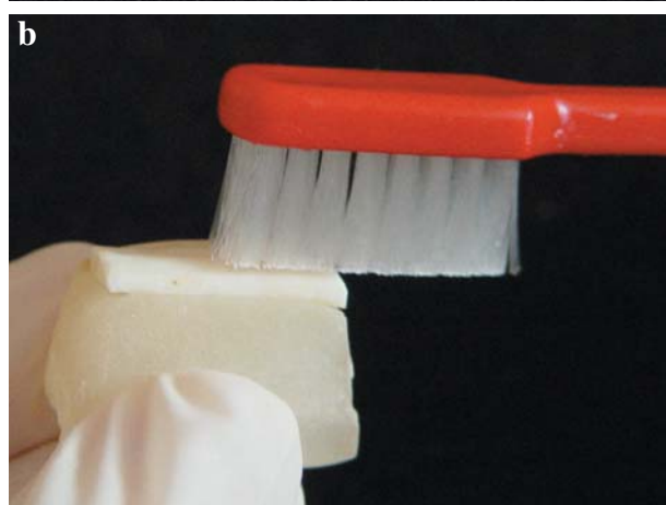
Figure 1- Bovine premolar tooth, and enamel surface fixed on an acrylic resin block (a) to facilitate the seizing for brushing (b)
