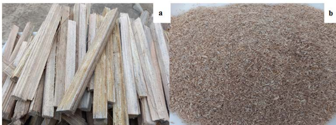
Figure 1 - (a) Miriti petiole structure and (b) miriti particles to produce panels
