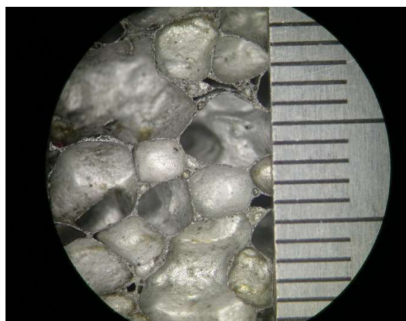
Figure 6: Mesoscopic structure of metal foam
