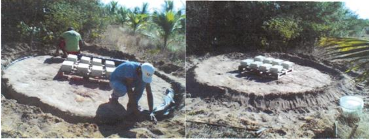
Figure 3 - Marking out the experimental plot for the instantaneous profile test
