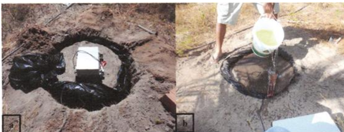
Figure 2 - Calibration of the sensor in the field: a – marking out the area to be used; b - saturation of the area
