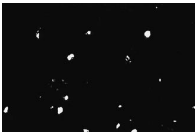
FIGURE 3 - Image obtained after processing of the digital image, 200 X. Total area is equal to 1.903 \times 10^6 \mu\text{m}^2 . The \text{Al}_2\text{O}_3 particles (clear spots) occupy 1.3 \times 10^4 \mu\text{m}^2 (0.7%).
