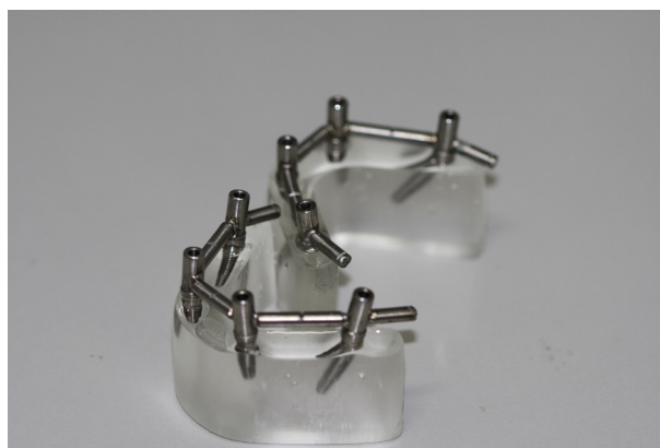
Figure.1: Photoelastic model (GIV Flexible Silicone Rubber and ASB - 10 Blue - POLIPOX®).
