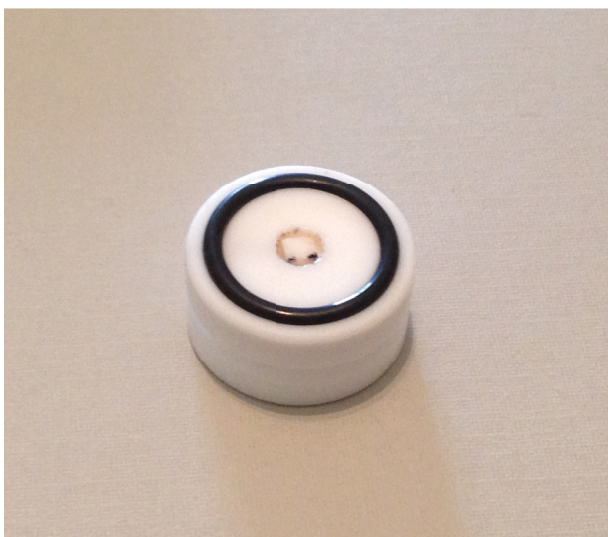
Figure 1. Acrylic apparatus where the dental enamel block was placed at the center.
