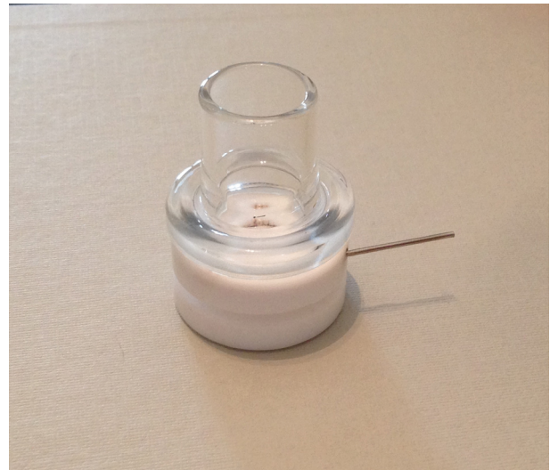
Figure 2. Glass apparatus placed over the acrylic apparatus, where 2 g of the formulation was added. At the side of the acrylic apparatus, there was an orifice, where the silver wire was placed, getting into contact with the side of the dental block.
