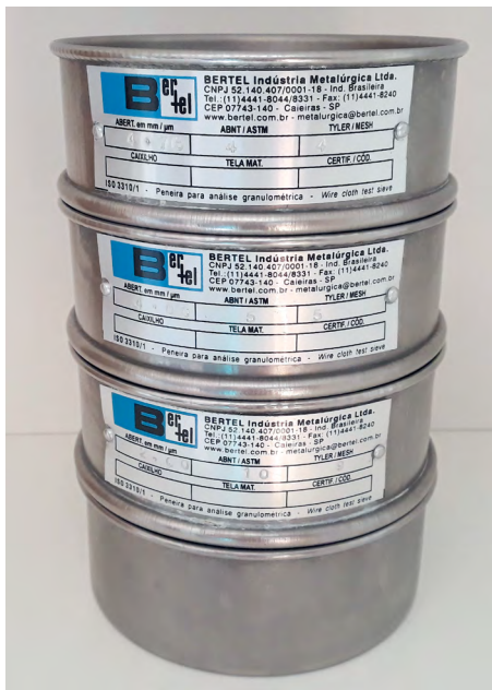
Figure 5. Sieving system vertically disposed for testing. The sieve with larger mesh spaces was placed higher, and that with smaller mesh spaces, at the bottom.
