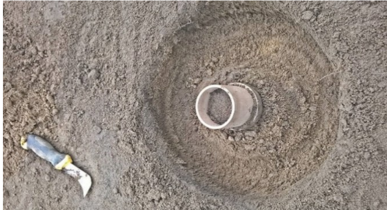
Figure 1. Physical collection of the soil samples using a soil auger with an internal PVC cylinder, to guarantee the preservation of the original structure of the soil in PVC cylinder for tomography analyses.
