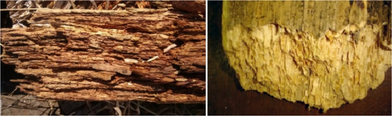
Figure 2. Wood attacked by soft-rot fungi, at advanced deterioration stages.
