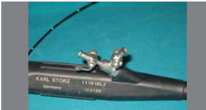
Figure 3. Manipulation channels of the thecaloscope (diameter 1.2 mm).
