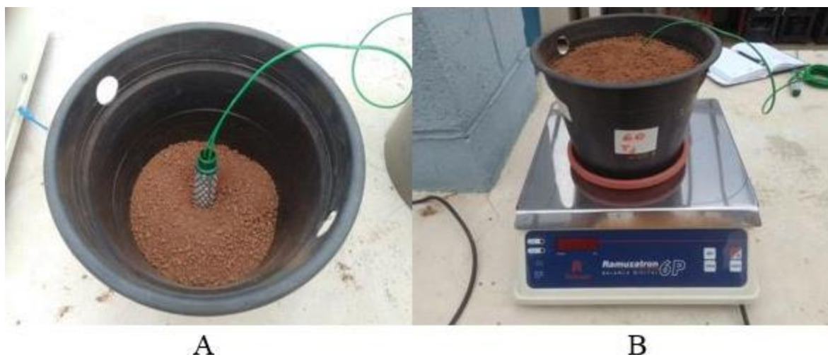
Figure 2. (a) Procedure of installation of the Watermark™ sensor in the pots and (b) daily determination of the wet weight of the soils of the experimental area to obtain the retention curves.
