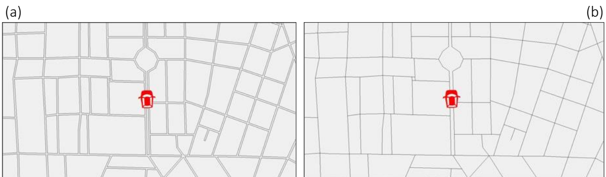
Figure 4: Map of 1:6,000 scale before (a) and after (b) application of collapse operator on road network.
