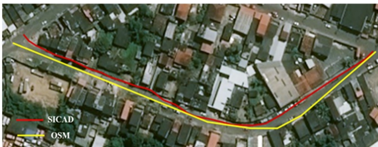
Figure 7: Linear Example 1 OSM linear features evaluated in relation to the Salvador Geodatabase.
