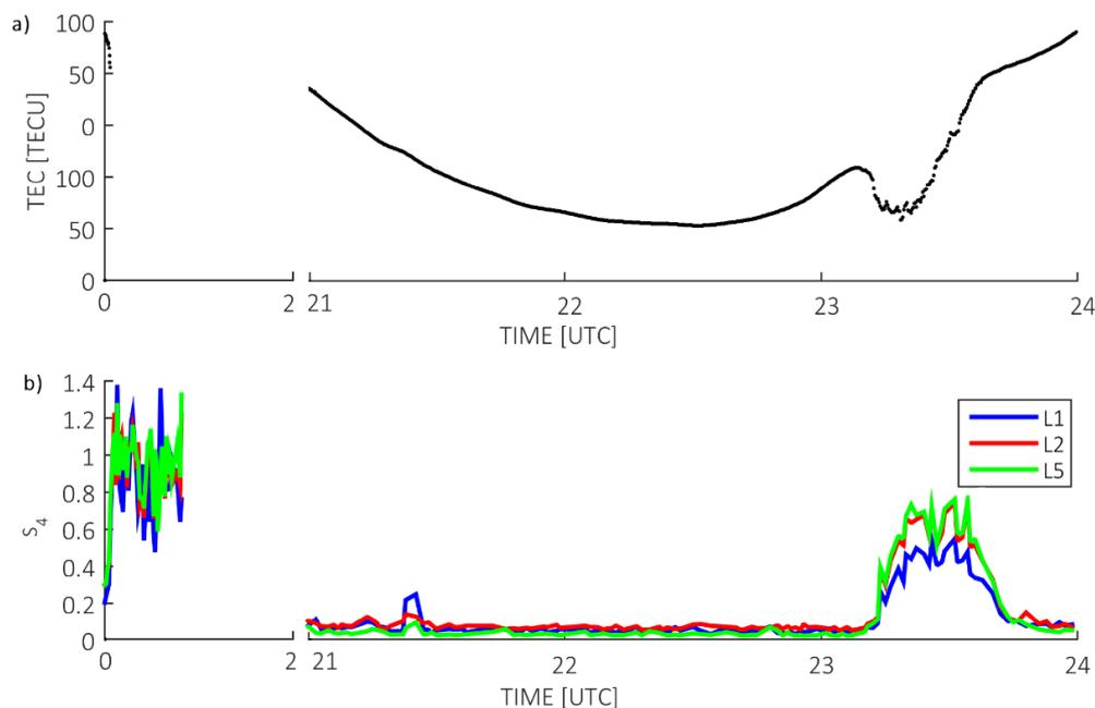
**Figure 2:** a) Slant TEC estimated for PRN 25 on November 27, 2014; b) The corresponding  $S_4$  values for L1, L2 and L5 signals.
