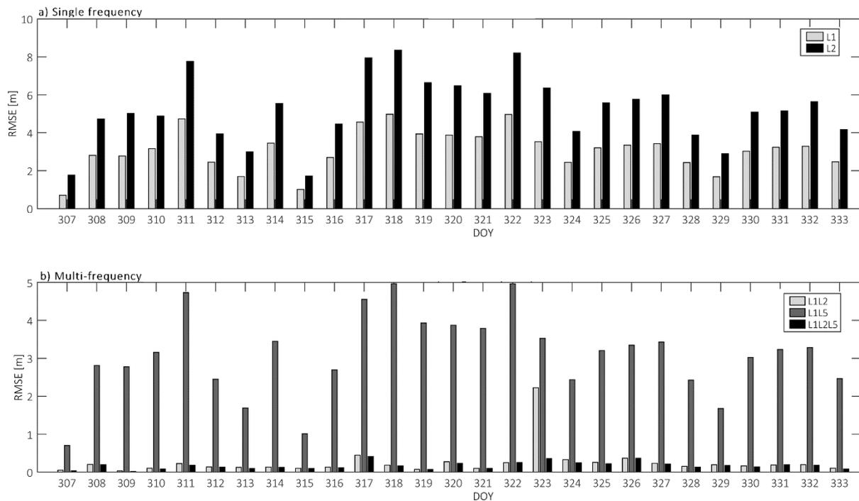
**Figure 4:** RMSE results for PPP processing considering different configurations, for SJCE station level (a) single frequency: L1 (light grey color) and L2 (dark color); (b) multi-frequency: L1-L2 (light grey color), L1-L5 (dark grey color) and L1-L2-L5 (black color).
