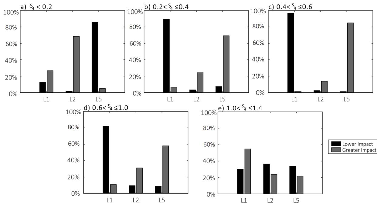
**Figure 3:** Percentage of epochs in which the GPS frequencies suffered least and highest impact considering  $S_4$  classification level (a) undisturbed level; (b) weak level; (c) moderated level; (d) strong level; and (e) saturated level.
