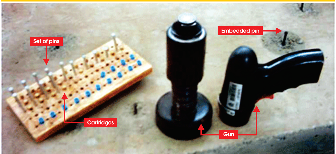
Figure 2 - Equipment used in the probe penetration test: gun, pins, and cartridges (gunpowder)
