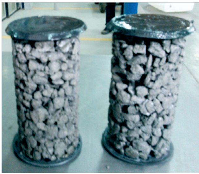
Figure 1 – Typical aspect of pervious concrete
