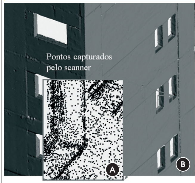
Figure 2 – (a) Illustration of a cluster of points captured by the scanner (Source: T1 Engenharia); (b) 3D model processed from the cluster of points captured by the scanner
