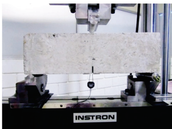
Figure 1 Three-point bending test (EN 14651 [7]) with measures in mm
