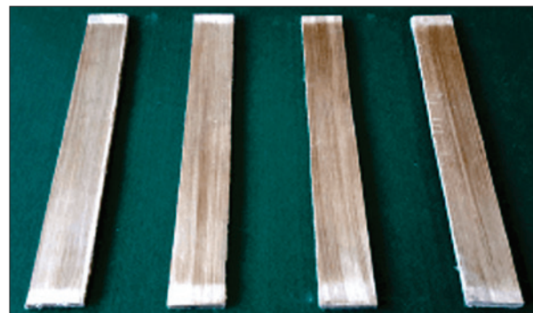
b) Reinforcement ready to gluing on the beams
