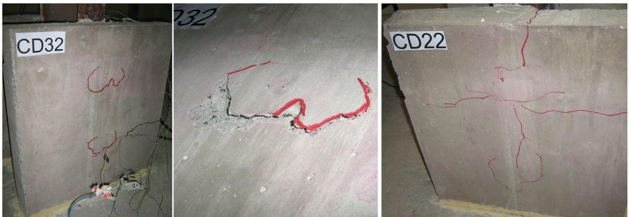
**Figure 17.** Cracks on push-out models' slab.
