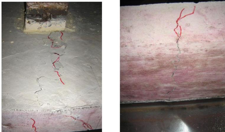
**Figure 18.** Beam V1A rupture configuration.
