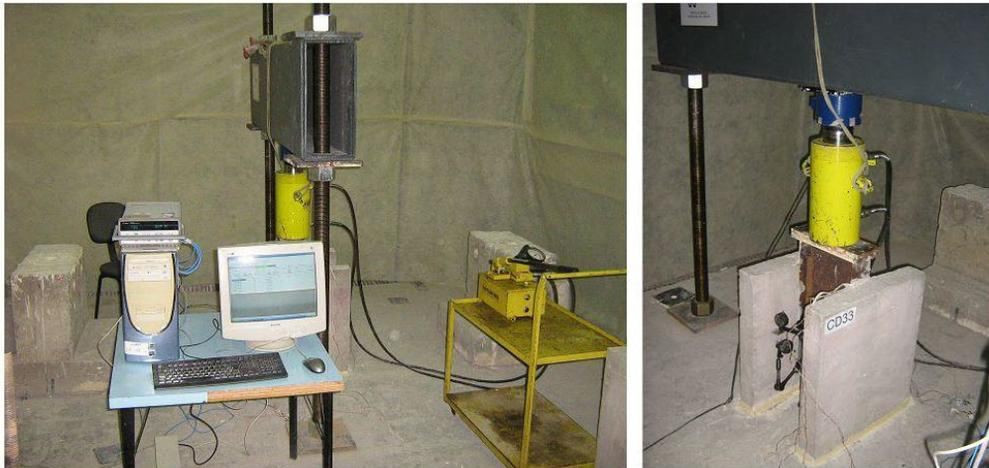
Figure 8. Test scheme for push-out.
