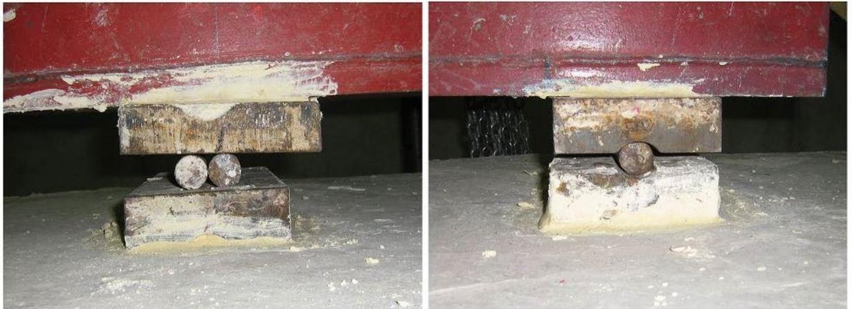
Figure 15. Load transmission beam support.
