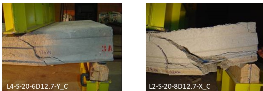
Figure 11. Hollow core slabs submitted to the shear test [17].
