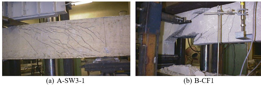
Figure 15. Failure modes observed in the beam tests [19].
