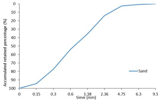
**Figure 1.** Sand's granulometric curve
