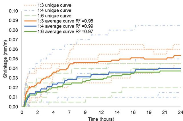
**Figure 11.** Early shrinkage curves of cement mortars sealed with PVC film. NOTE: dotted lines indicate individual tests, continuous ones are their respective average curves and their legend contains their linear R used to find shrinkage speed.
