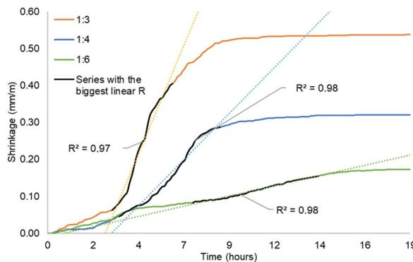
**Figure 10.** Average early shrinkage curves of exposed to air samples and their selected series for shrinkage speed calculation. NOTE: time scale of the graph used in 19 hours to improve the visualization of the selected series for calculating the intermediate stage’s slope. The dotted lines represent the linear trend line taken from the series with the highest linear R within the intermediate stage.
