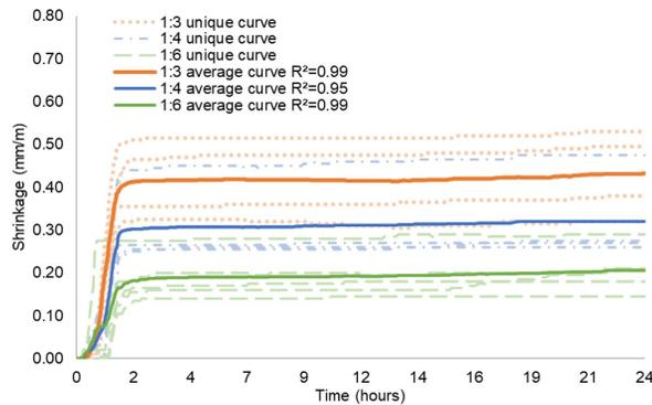
**Figure 12.** Early shrinkage curves of cement mortars exposed to 5 m/s wind. NOTE: dotted lines indicate individual tests, continuous ones are their respective average curves and their legend contains their linear R used to find shrinkage speed.
