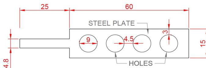
**Figure 2.** Rigid element vertical view (measurements in mm)
