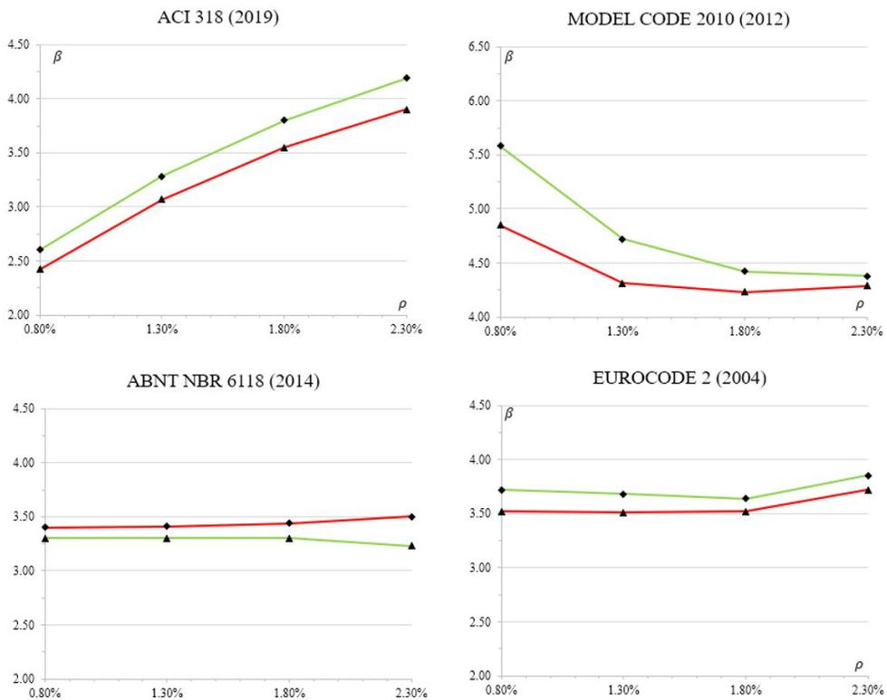
Figure 7. Reliability index bounds of code designed as function of reinforcement ratio
