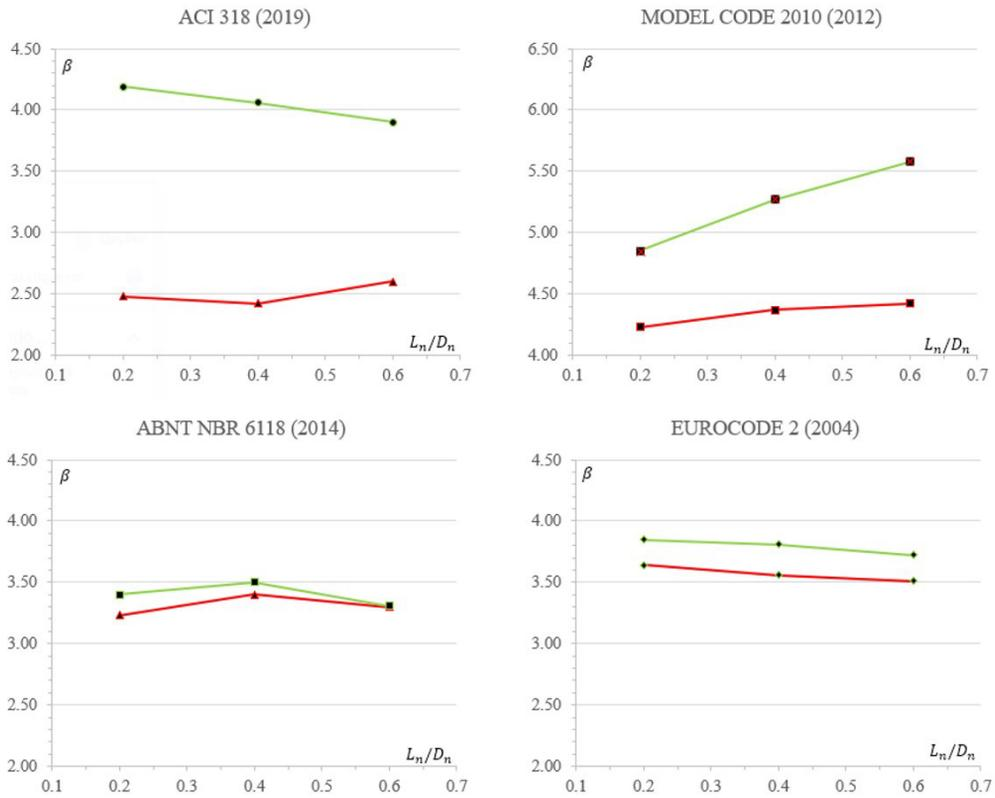
Figure 6. Reliability index bounds of code designed as function of load ratio
