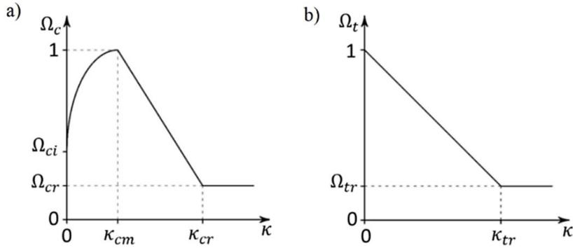
Figure 1. Hardening and softening functions in compression and tension [10]
