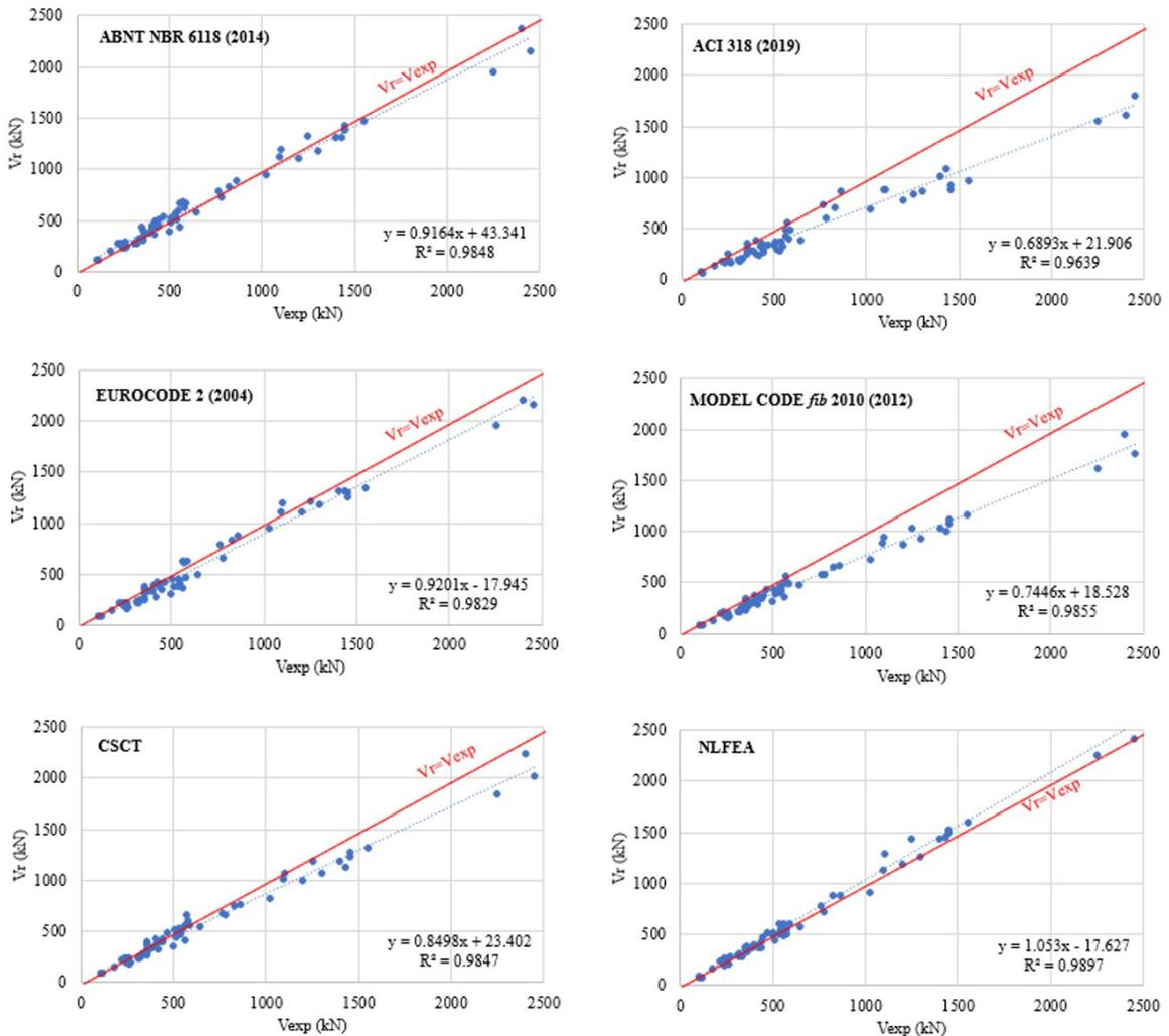
Figure 3. Relation between experimental and predicted value of punching shear strength
