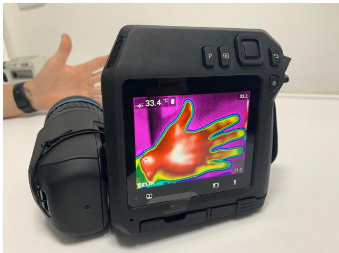
Figura 2. Termocâmara Flir® modelo T540sc (Flir Systems Inc, Wilsonville, OR).
