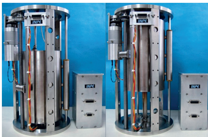
Figure 2. Solidification furnace in its two working phases: positioned at the bottom, heating the sample during ground and ascending period, and dislocated to the top permitting a fast sample cooling during microgravity.
