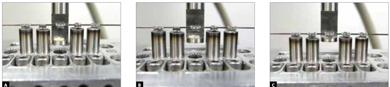
Figure 3 - A) Inferior displacement of the support and application of composite resin. B) Support rising. C) Placement of the canine bracket in a passive configuration.
