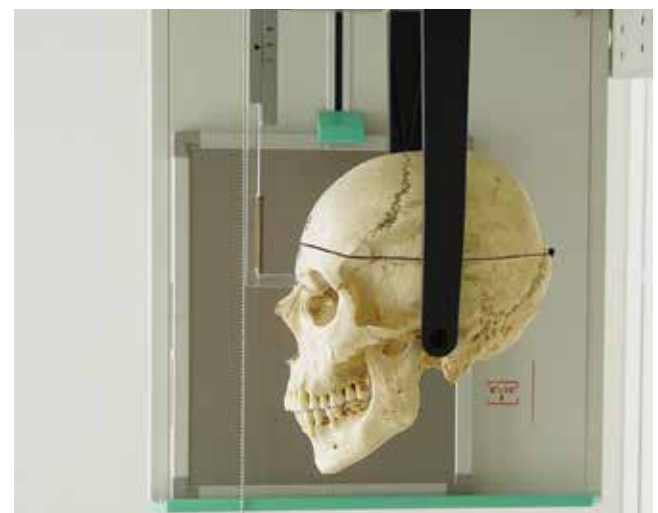
Figure 2 - Positioning the skull on the cephalostat.
