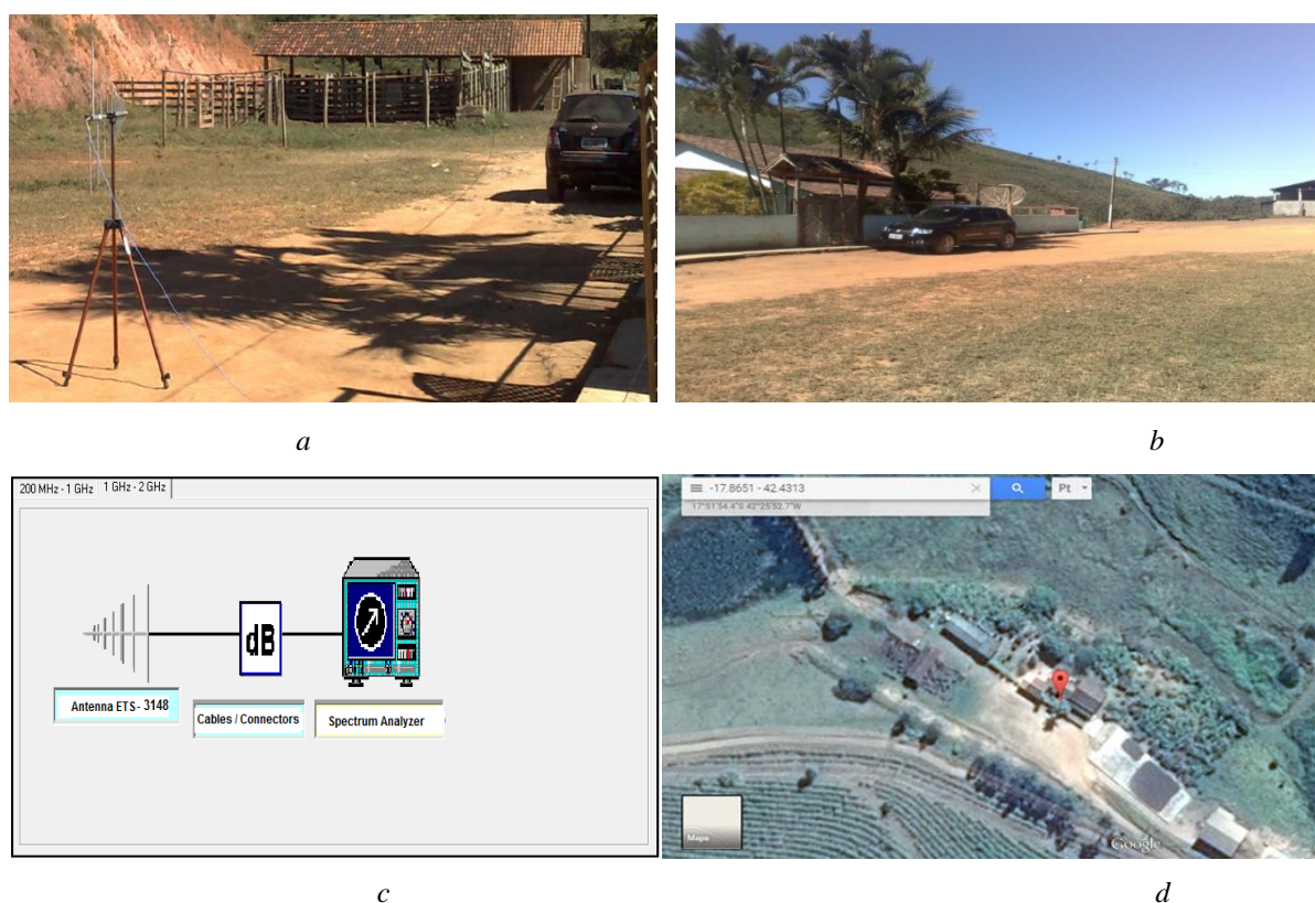
Fig. 1. Log-Periodic Dipole Array Antenna, the parking near the city of Capelinha, aerial photograph and the setup used: (a) Antenna – 3148; (b) Parking located at Lat. 17.8651°S Long. 42.4313°W; (c) Setup used to measure the electromagnetic noise in open area; (d) Farm located near the city of Capelinha, state Minas Gerais, Brazil (Lat.17,8651°S – Long. 42,4313°W) [Reference source: Google maps]
