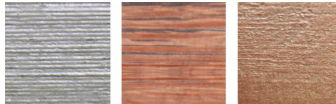
Fig. 7. Details of surface of the horns coated with silver paint, copper tape and copper plated.
