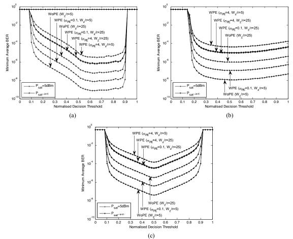
Fig. 3 Minimum average BER over a range of normalised decision thresholds WoPE  $(W_z/r \in \{5, 25\})$  and WPE  $(\sigma_{PE} \in \{0.1, 4\}, W_z/r \in \{5, 25\})$ ; including GS, PE and AT effects.  $P_{sat} \in \{5dBm, \infty\}$ (a) SPA (b) GA (c) MCB
