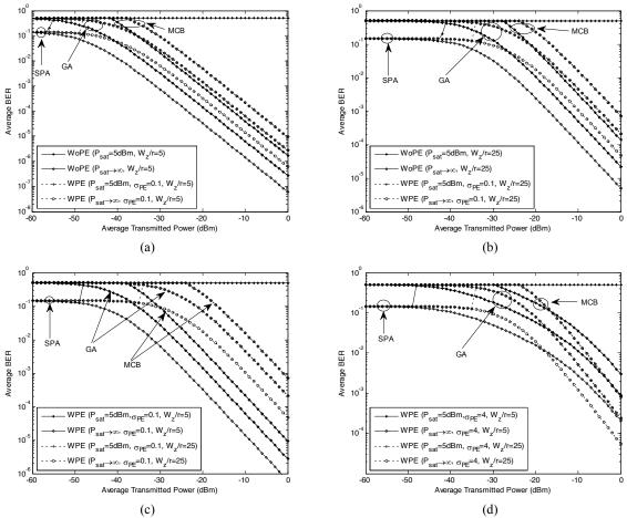
Fig. 2 Average BER over a range of average transmitted powers for SPA, GA and MCB performance evaluation methods; including GS, PE and AT effects.  $P_{sat} \in \{5dBm, \infty\}$
