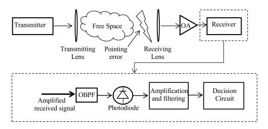
Fig. 1. FSO communication system model with PE and a preamplified optical receiver
