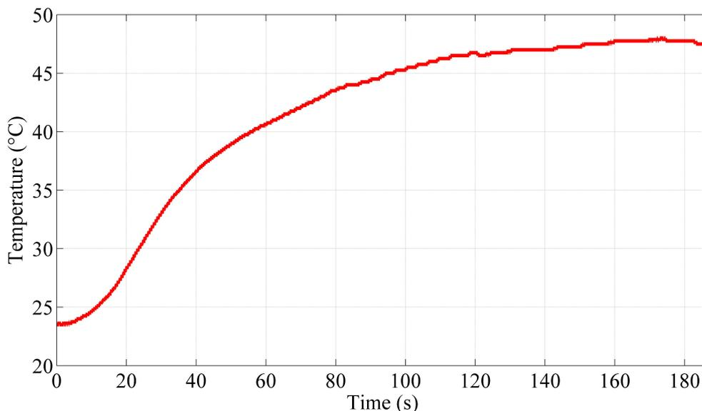
Fig. 4. Temperature measurements acquired from the PoF-powered 433-MHz wireless sensing system over 3 minutes.
