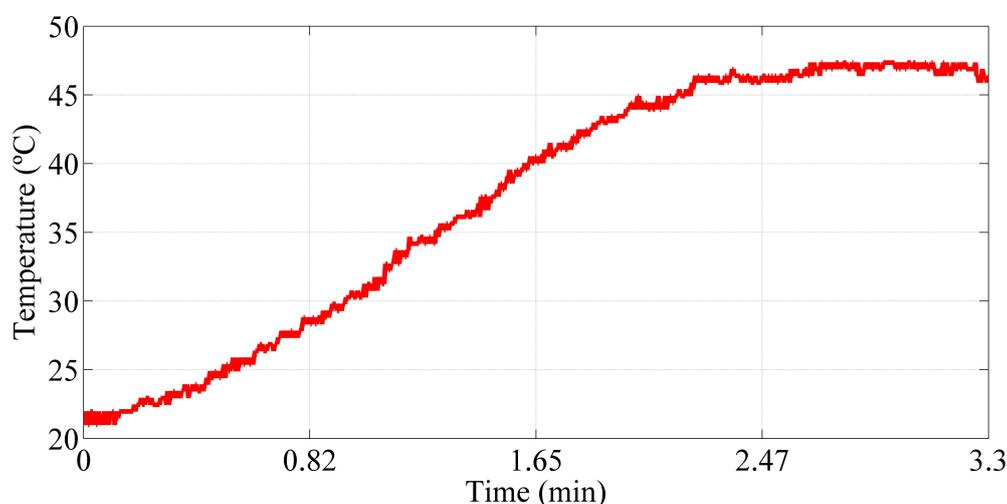
Fig. 7. Temperature measurements acquired from the PoF-powered 2.4-GHz wireless sensing system over 3 minutes.
