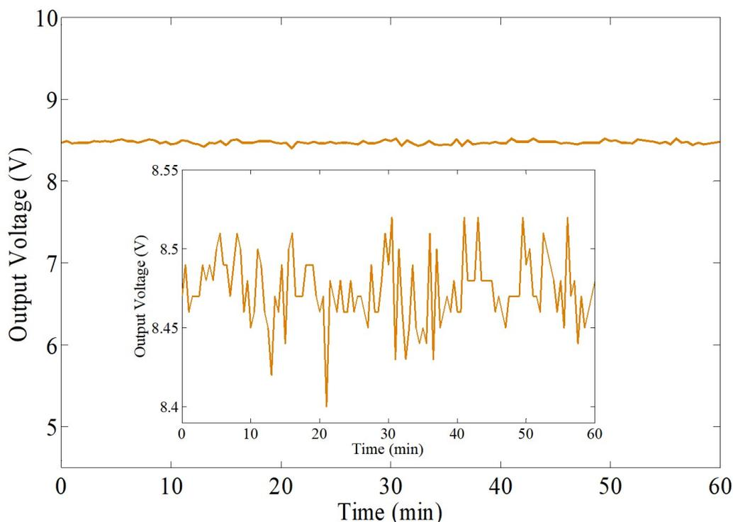
Fig. 3. PoF system output voltage measurements over a 60-minute period.
