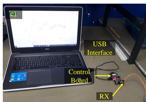
Fig. 5. Second implemented PoF-based wireless sensor system: a) Block diagram, b) Experimental setup photograph of the PoF system, control board, and 2.4-GHz transmitter, c) Experimental setup photograph of the reception side, including the control board, receiver and computer.
