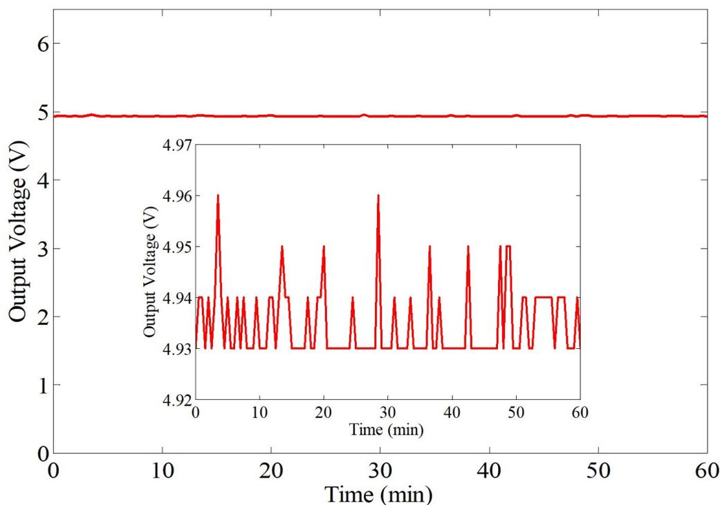
Fig. 6. PoF system output voltage measurements over a 60-minute period using a DC/DC converter.
