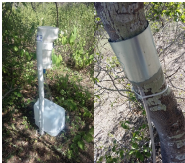
Figure 2. Measurement of throughfall (left) and stemflow (right) in plant species of the Caatinga domain in municipality of Floresta, State of Pernambuco, Brazil.
