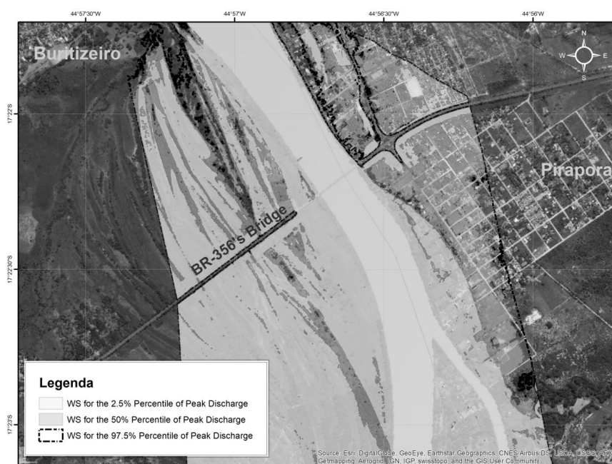
Figure 7. 1992 flood probabilistic inundation map in the upstream portion of Pirapora.
