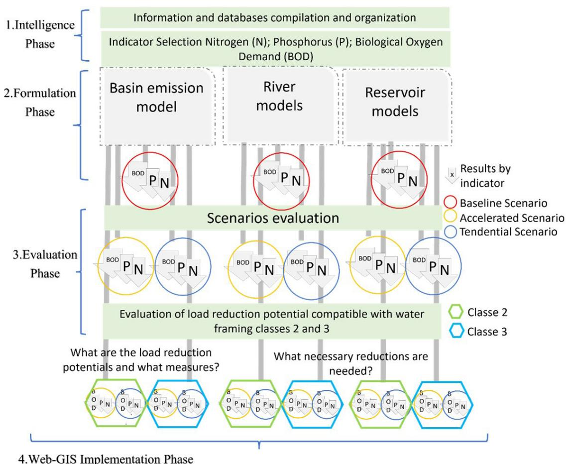
**Figure 2.** Phases of data processing and modeling necessary to implement the Web-GIS.
