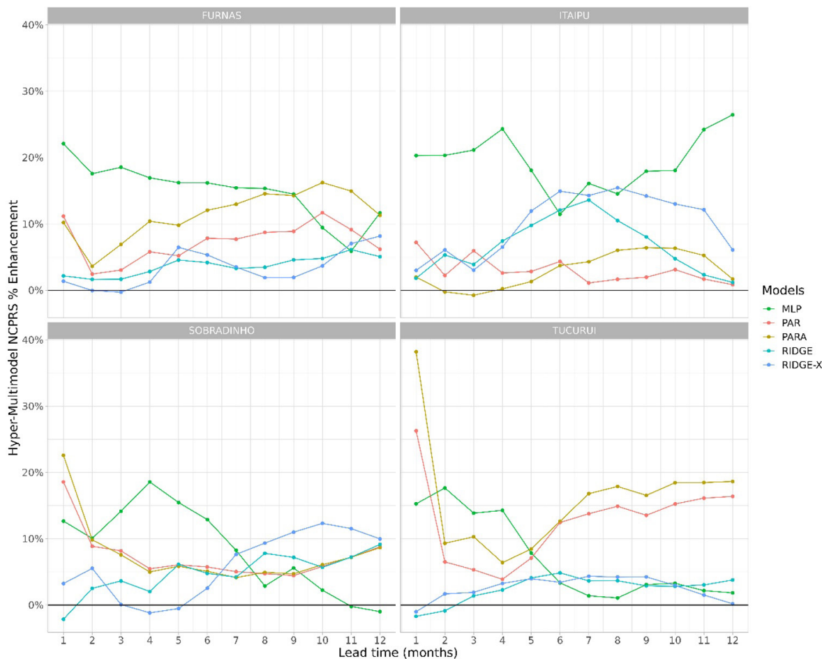
Figure 7. Normalized Continuous Ranked Probabilistic Score (NCRPS) percentage enhancement of the Hyper-Multimodel in comparison to individual models for lead times from 1 to 12 months for the 4 key stations - Calibration Period (2001 to 2010).
