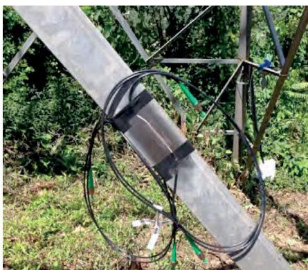
Figure 8 Optical sensor installed in the structural element and the system power set.
