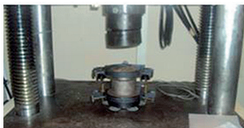
Figure 5 Piston-die system used in the compression tests.
